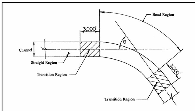
Figure 3-2: Channel bend region (from AASHTO LRFD Figure 3.14.5.2.3-1b)
