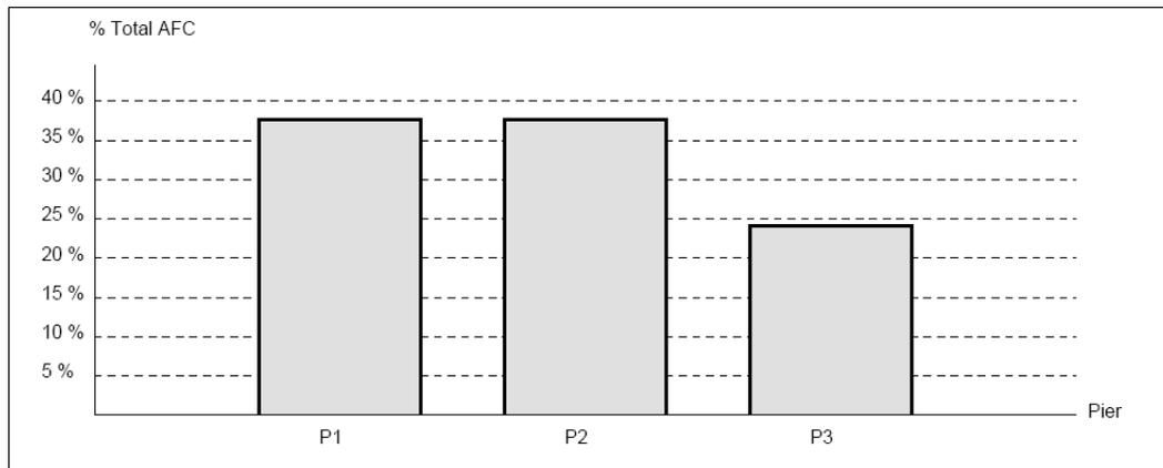
**Figure 6-13: Contribution towards the annual frequencies of collapse of all vessels passing a particular pier of the San Jacinto River – EB IH 10 Bridge (from the VIOB Report)**
