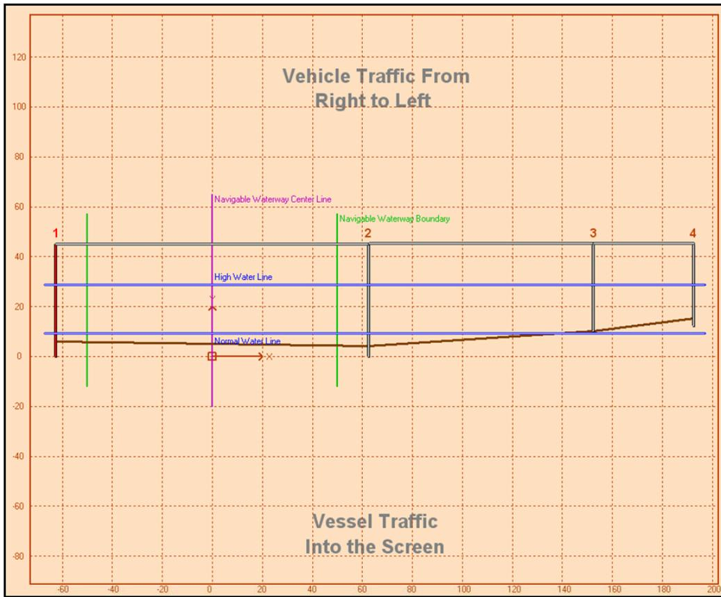
**Figure 5-1: Colorado River – FM 521 Bridge Geometry.**
