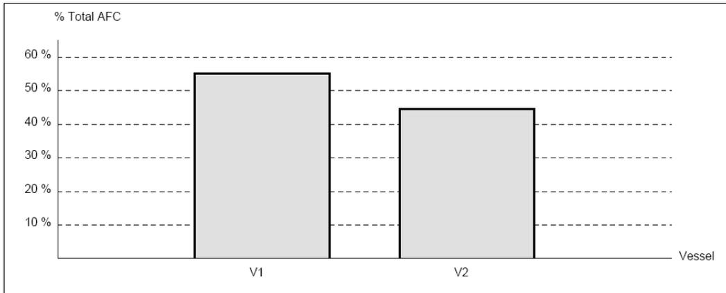
**Figure 6-12: Contribution towards the annual frequencies of collapse of a particular vessel passing all piers of the San Jacinto River – EB IH 10 Bridge (from the VIOB Report)**
