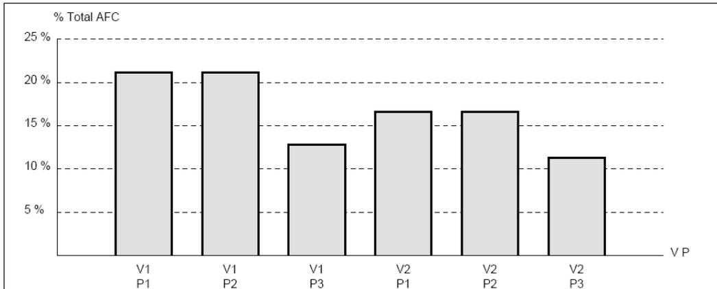
**Figure 6-11: Contribution towards the annual frequencies of collapse of a particular vessel passing a particular pier of the San Jacinto River – EB IH 10 Bridge (from the VIOB Report)**
