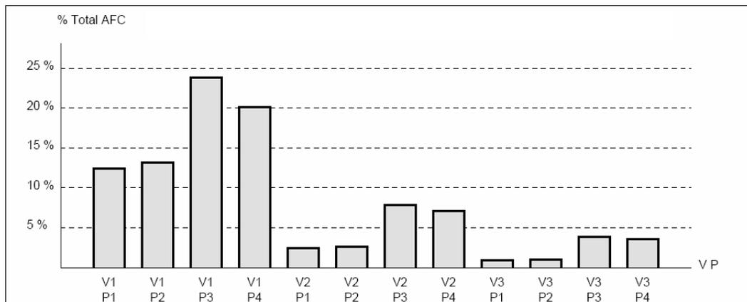
**Figure 6-4: Contribution towards the annual frequencies of collapse of a particular vessel passing a particular of the Colorado River – FM 521 Bridge (from the VIOB Report)**
