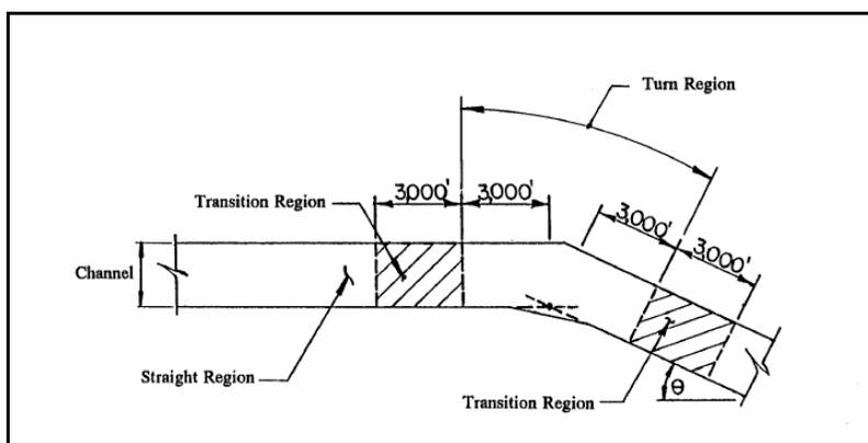
Figure 3-1: Channel turn region (from AASHTO LRFD Figure 3.14.5.2.3-1a)
